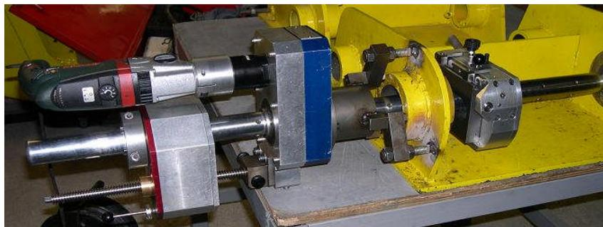
*This attachment needs no other motor than the one of the portable boring bar.*
